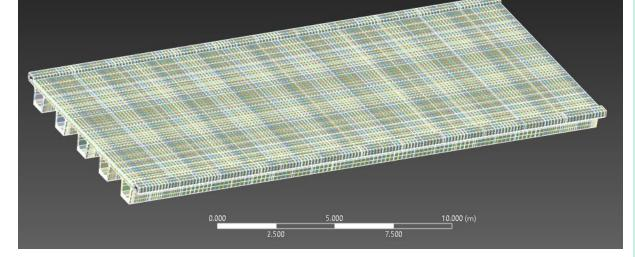
Digital 3D section of the two concrete bridges by using over 1.07 million points obtained from the Terrestrial Laser Scanning visualising all surfaces of the concrete bridges. The 3D visualisation demonstrates the surface defects which might not be detected by the FE model. These defects might come from the environmental impacts that causes the structural deterioration of trafficking impacts such as the potholes or rutting.
